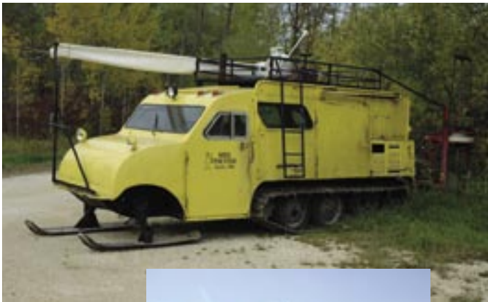
Getting to where the fish are: the odd-looking vehicle to the left is a Bombardier Muskeg , used on snow and ice and equipped with an ice auger that is used for winter fishing; below, a more identifiable form of transportation: Karen's brother Kris aboard his fishing boat at dockside in Gimli.
